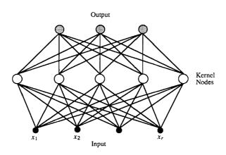
Figure 1: A radial-basis-function network.
